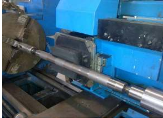
Roll undergoing EDC texturing
